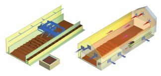
**Waste is inserted**. Up to 25 cubes of waste a day, consisting of excrement from one or several types of animals, is placed in the fermentation area. Liquid waste, like that of pigs, may be supplemented with organic material that absorbs water, resulting in a more solid product. Any organic matter in the form of wastage may also be added.
